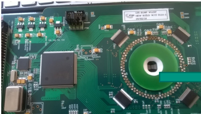
Probe Card Tester for Belle 2 (ASIC in AMS 180um HV process)
